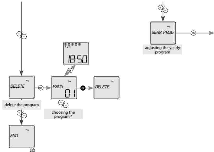
\* By shortly pressing **OK**, you can toggle between the program number and the display of its settings. Use **%** to toggle preset programs. By holding **OK** you can proceed with the required step - *CHANGE / DELETE*. If you do not want to proceed, press **ESCAPE** to go to the main settings without any change.
