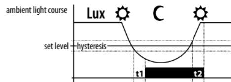
t1 - delay time when switching on
