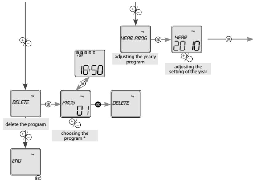
By shortly pressing **OK**, you can toggle between the program number and the display of its settings. Use **%** to toggle preset programs. By holding **OK** you can proceed with the required step - **CHANGE / DELETE**. If you do not want to proceed, press **ESC** to go to the main settings without any change.
