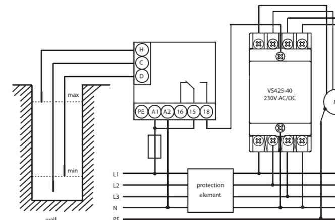
Monitoring TWO LEVELS minimum / maximum - DRAINING function - (PUMP DOWN)
