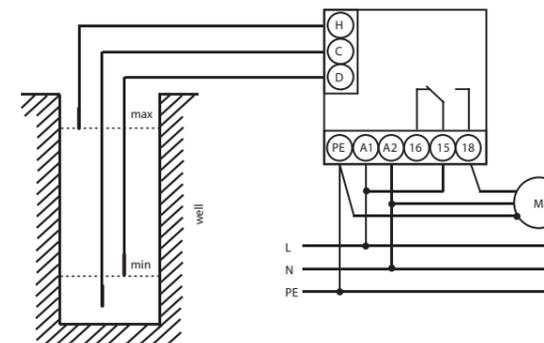
Monitoring TWO LEVELS of the FLUID LEVEL minimum / maximum - DRAINING function - (PUMP DOWN)
