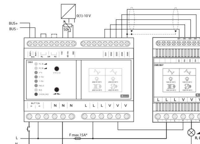
\* Potential L on device terminal, has to be protected by circuit breaker accordant to the load connected to device.
