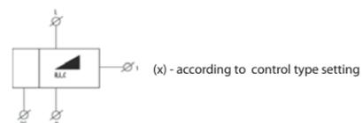
\* Warning : it is not allowed to connect inductive and capacitive loads at the same time.
